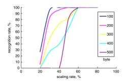
Fig. 3 Scaling and recognition rates of multi-view QR code
