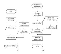
Fig. 2 Flowchart of multi-view QR code a Encoding b Decoding
